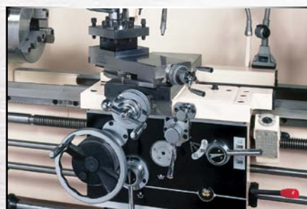
Carriage Features One-Shot Lubrication and Turcite B on Sliding Surfaces
